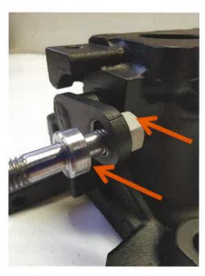
After loosening the self-locking nut together with the washer, simply move the lever and tighten the nut.
